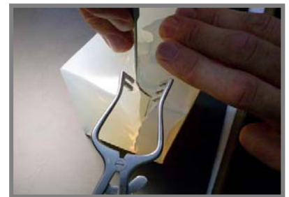
Figure 7 Pouring the mixed silicone rubber
