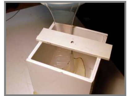
Figure 7 Pouring the mixed silicone rubber
