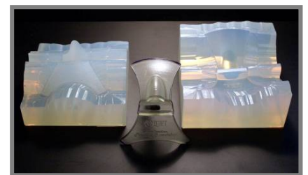
Figure 9 Master model and silicone mold
