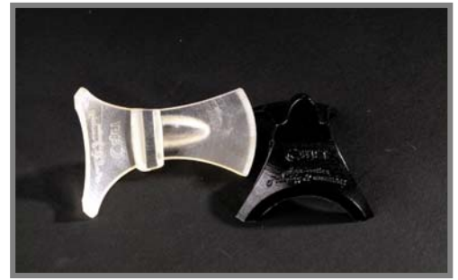
Figure 11 Illustrated above: a final part (black) and its master model. Information and photos courtesy of Varinex/ Hungary.
