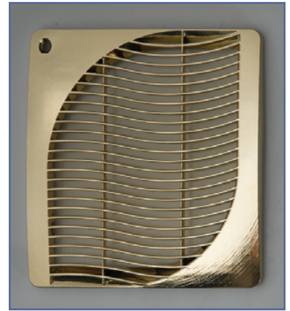
Picture 4. PolyJet model coated with gold finish
