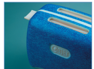
Picture 4. Example of textured PolyJet model.
