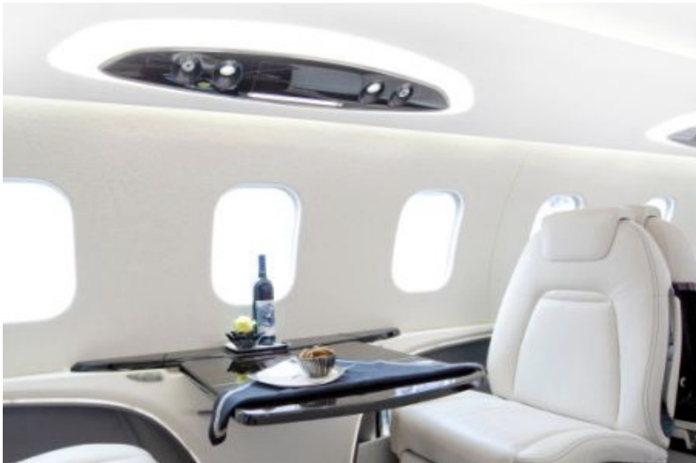
Prototypes of the Learjet 85's passenger service units, which house LEDs and oxygen masks, were created using Objet's rapid-prototype equipment.
